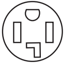
4-wire receptacle (14-30R)
