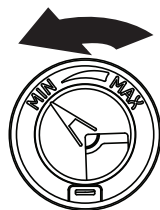
Counterclockwise to reduce foaming
