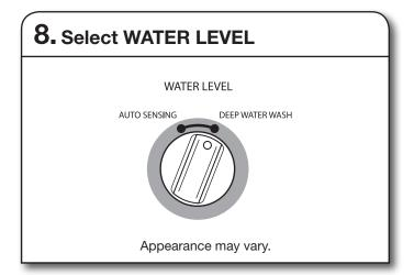
Set the Water Level knob to the Auto Sensing setting and the washer will fill to a level that ensures the load engages the agitator. From this point, the electronic control will sense the load and determine if additional water is needed. Select Extra Rinse for enhanced rinsing performance.
