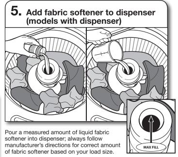
Dilute liquid fabric softener by filling the dispenser with warm water until liquid reaches the underside of the rim. See Max Fill line arrows.
