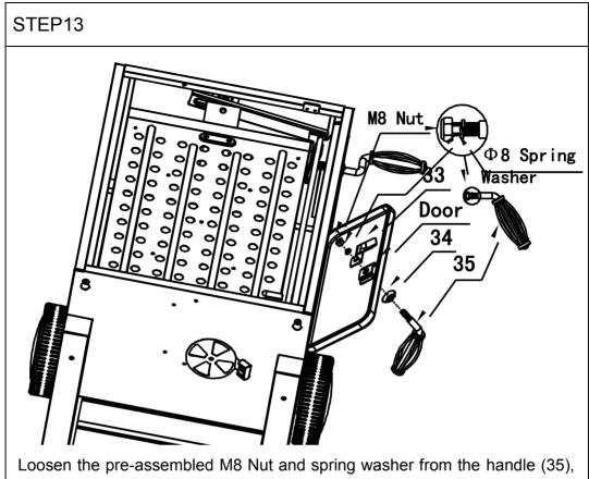
and then assemble the handle to Charcoal Door according to the diagram as shown.
