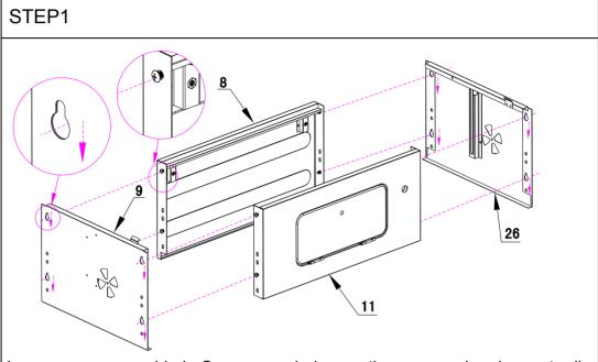
Loosen pre-assembled Screws and leave the screw heads protruding approximately 5mm. Hang the side panels onto the screws and tighten them.
