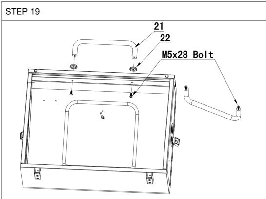
Loosen the pre-assembled M5x28 Bolts from Hood Handle (21), and then assemble the handle together with spacer (22) to the hood according to the diagram as shown.
