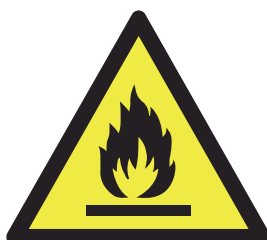
Caution: Risk of fire/ flammable materials
