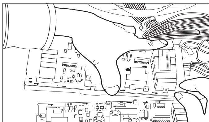
Figure 4-18. Light Transformer Removal.
