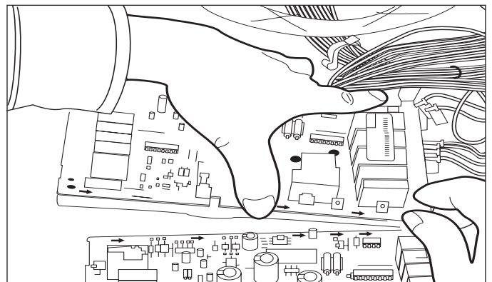
Figure 4-18. Light Transformer Removal.
