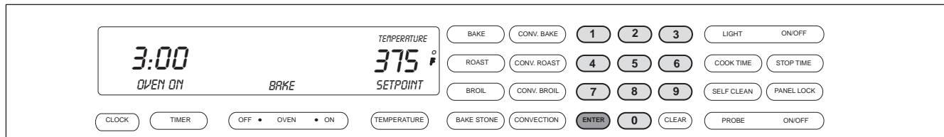
Figure 3-25. To change the preset temperature, immediately press the number keys to enter a new temperature. Then, press the ENTER key.
