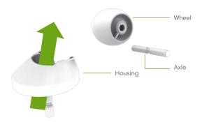
Important: A front wheel clogged with hair and debris could result in floor damage.
