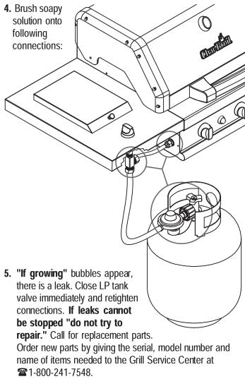
**6.** Always close LP tank valve after performing leak test by turning hand wheel clockwise.
