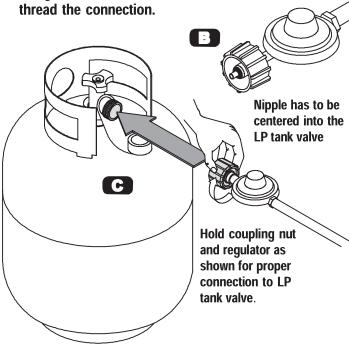
6. Turn the coupling nut clockwise to tighten to a full solid stop. The regulator will seal on the back-check feature in LP tank valve, resulting in some resistance. An additional one-half to three quarters turn is required to complete connection. Tighten by hand only - do not use tools.
