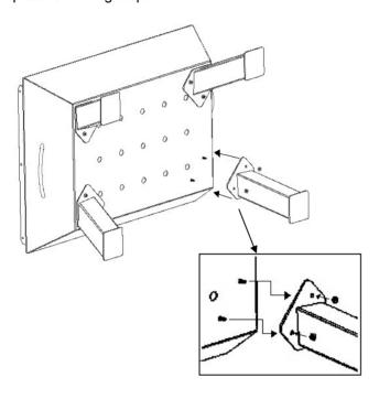
**STEP 2.** Attach 1 side panel to each short end of firebox using 3 #10-24 x 1/2" Combo truss head screws from the outside of firebox and attach 3 #10-24 KEPS nuts to screws from the inside. Tighten all screws and nuts.
