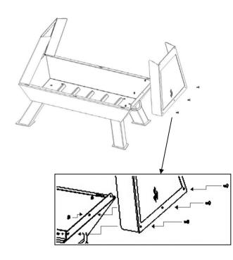
**STEP 3.** Set the top cap assembly down onto the side panels. Make sure the side panels are on the outside of the top cap mounting flange. Attach top cap using 2 #10-24 x 1/2" Combo truss head screw per side and 2 #10-24 KEPS nuts. Attach screws from outside of fireplace (as shown). Tighten all screws and nuts.
