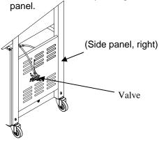
Step 3: Insert valve stem assembly into burner venturi.
