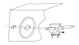
Step 8: Place knob on valve stem and secure with wrench.
