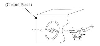
Step 6: Align & tighten knob bezel & valve stem with 2(two) screws & washers as shown below.
