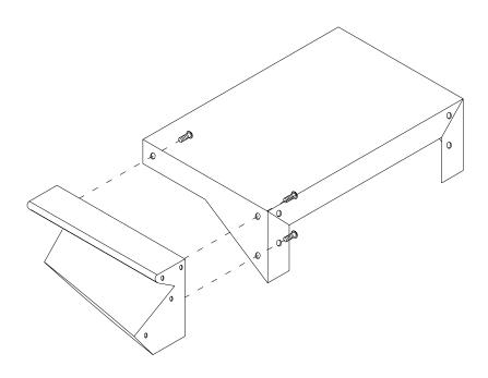
Step 11: Assemble the panel of side burner with three(3) pcs 1/4\*12 screws as shown figure below.
