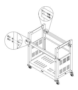
**Step 5:** Insert fix piece of door shaft into the square pipe at left and right side as shown figure below, screw four(4)pcs 5/32\*12 screws. Attention: Do not screw too tight.
