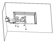
Step 7: Tight all 4(four)screws on the "U" brackets on the burner, then connect the ignition wire on to valve.
