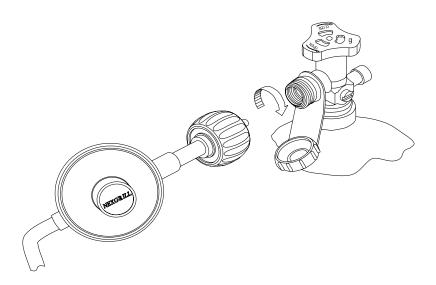
CAUTION! DO NOT USE TOOLS TO ATTACH REGULATOR / HOSE ASSEMBLY TO PROPANE TANK
