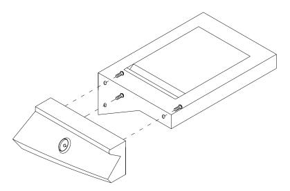
Step 12:. Assemble the side shelf and panel of side burner into the firebox with eight(8) pcs 1/4\*12 screws.
