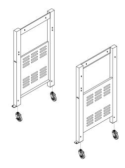
Step 2: : Assemble bottom panel to side panels with four (4) pcs 1/4\*42 mm screws as shown figure below
