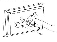
Step 4: Insert valve stem assembly into control panel.
