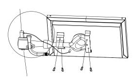
Step 2: Remove 4(four)screws & washer from the "U" . brackets on the side burner.
