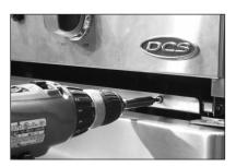
Secure grill to the front of the cart with Phillips-head screws (provided).
