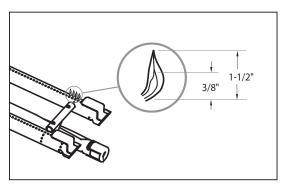
FIG. 07 Burner Flame Height
