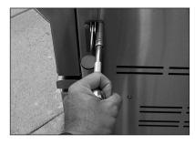
E) Install bolts omitted from Step 4 to secure grill body to the cart side for added strength.
