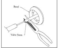
FIG.10 Low Setting Adjustment
