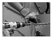
D) Secure grill to rear of cart with phillips-head screws (provided).
