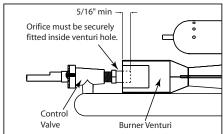
Be careful not to upset the air shutters' original position (unless readjusting). Lower the rear of the burner into the cutouts on the support channel at the rear of the burner box. Make sure it is level and does not rock. Light all of the burners and check for proper flame characteristics. If adjustments are necessary, refer to (page 14). Do this prior to cooking on the grill.
