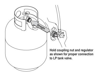
6. Turn the coupling nut clockwise and tighten to a full stop. The regulator will seal on the back-check feature in the LP tank valve, resulting in some resistance. An additional one-half to three-quarters turn is required to complete the connection. Tighten by hand only – do not use tools.
