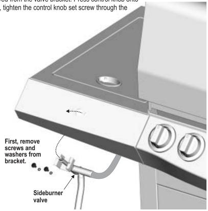
Insert sideburner into shelf, placing end of burner over sideburner valve. Valve should be in center hole of burner tube. Make sure pin on bottom of burner is in center hole in shelf bracket. Secure burner to bracket with two #10-24x3/8" screws (III), 5mm lock washers (JJJ), and 5mm flat washers (KKK). See illustration below for correct burner-to-valve engagement.
