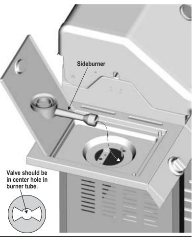
Insert valve clip into small hole in bottom of burner, then snap other end of clip over sideburner valve. Beneath sideburner shelf, attach sideburner ignitor wire to electrode. Place brass top on sideburner, then place sideburner grate onto shelf.
