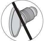
Do not use a POL transport plug (plastic part with external threads)! It will defeat the safety feature of the valve.
