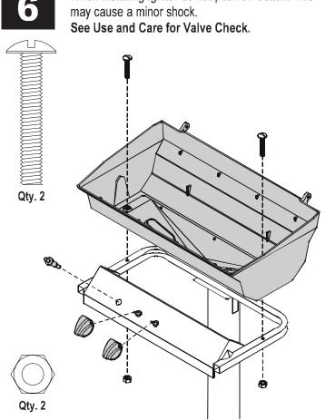
When installing Ignitor do not push on button. This
