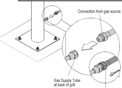
After connecting grill to gas line, perform leak test
